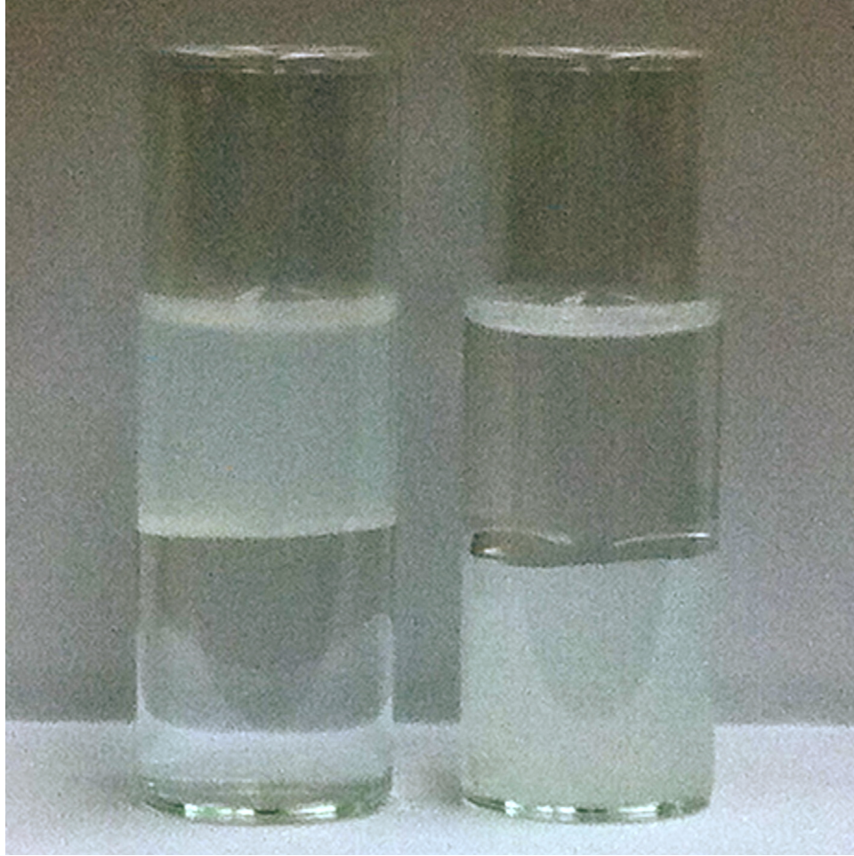
Figure 3.17. Organic capped ZnO particles are suspended in hexanes (left). MUA capped ZnO, after ligand exchange, are suspended in water (right).
